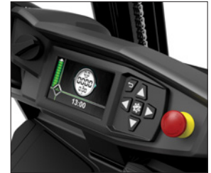
Multifunctional colour display (hourmeter, BDI etc.)
