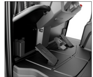
Dual pedal system - forward and reverse. (Option)
